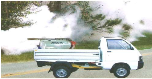
Figure- 31: Vehicle mounted fogging machine
